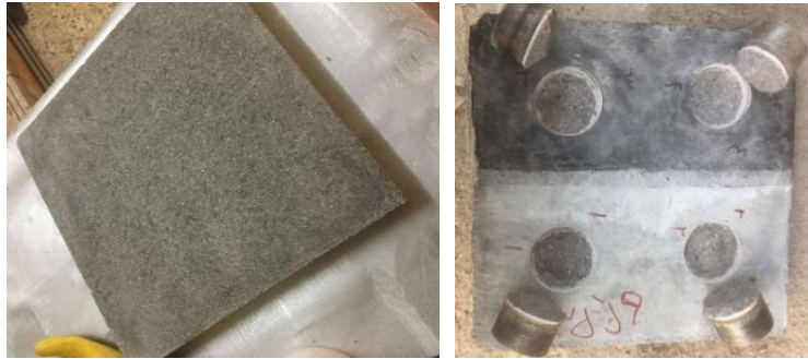
Fig. 6. High strength specimen and failure mode in second try test method
