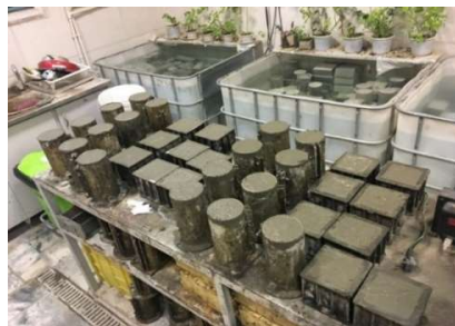
Fig. 1. The cubic/cylindrical concrete specimens
