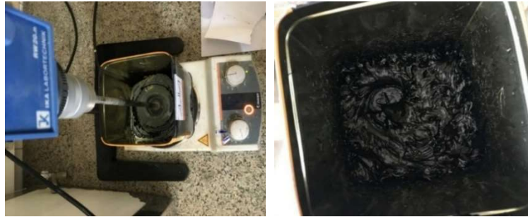
Fig. 2. a) mixing epoxy with CNTs (left), b) modified epoxy (right)
