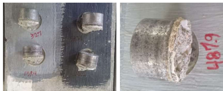
Fig. 5. Failure mode of the specimens in first pull-off test
