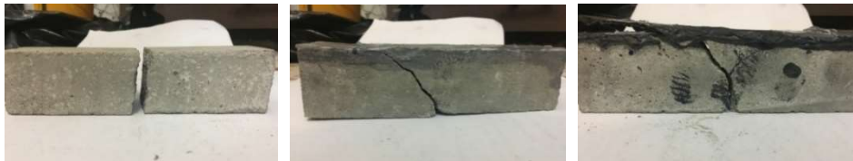
Fig. 14. Failure in the bending tests of SC, RCFRPSE, RCFRPM specimens, left to right, respectively
