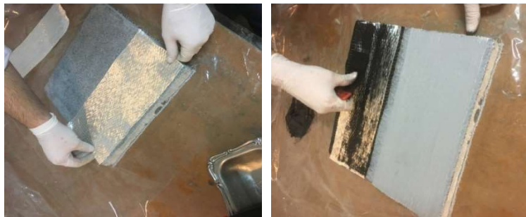
Fig. 3. Installation of FRP on the concrete sheets and removing air pockets by laminate roller
