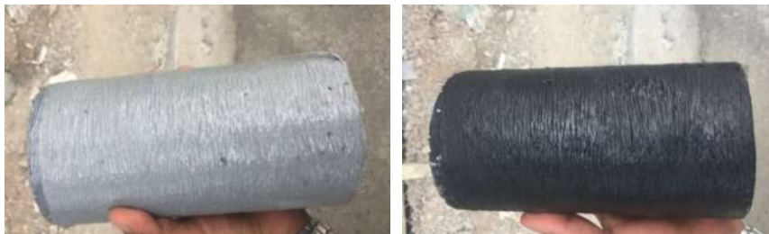
Fig. 8. Specimens for compression strength test: a) RCFRP (left), b) RCFRPME (right)
